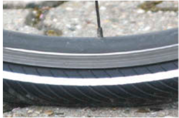
Figure 119: Correct tyre pressure. The tyre is barely deformed under the load of the body weight
