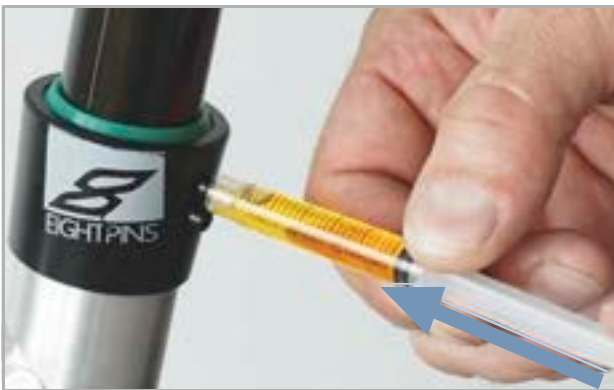
Figure 196: Lubricating the Eightpins seat post
