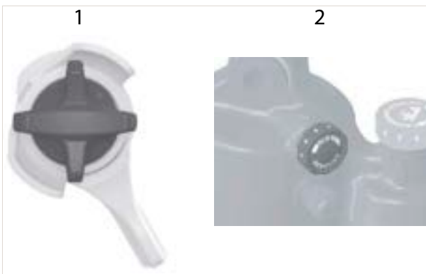
Figure 267: Float DPS (1) and Float X (2) rebound adjusters
