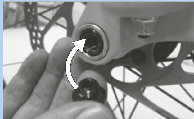
Figure 76: Inserting the securing screw
