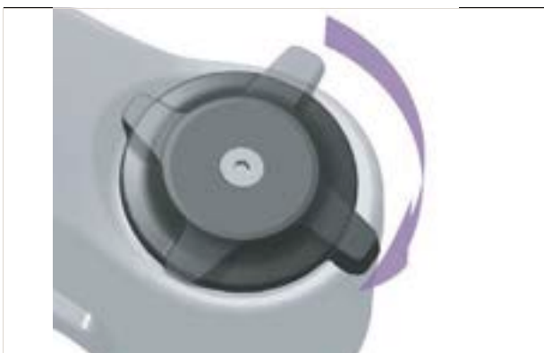
Figure 237: Adjust the compression adjuster so that it is harder
