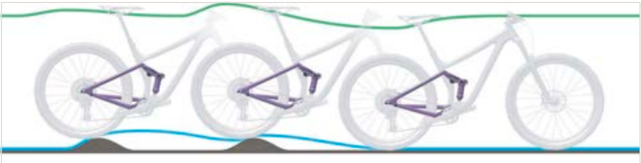
Figure 258: Rear frame damper rebounding too slowly
