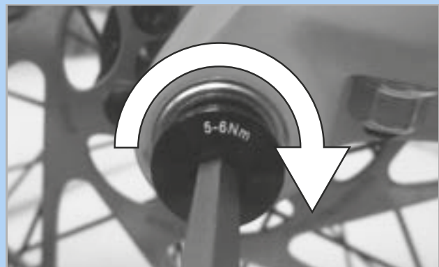
Figure 77: Tightening the securing screw
