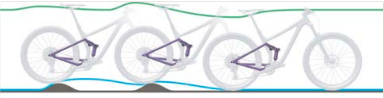
Figure 266: Rear frame damper rebounding too slowly
