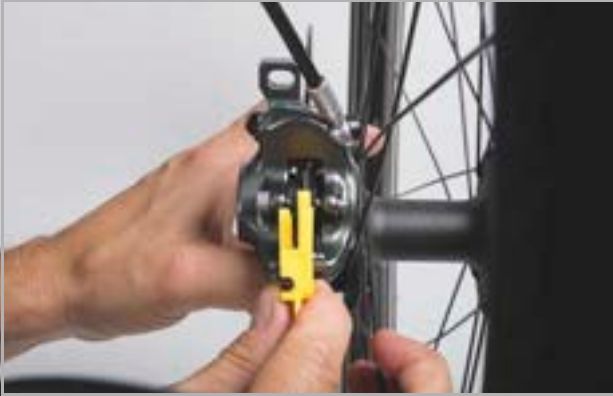
Figure 200: Checking the brake lining when fitted with the help of the transport safety wear gauge
