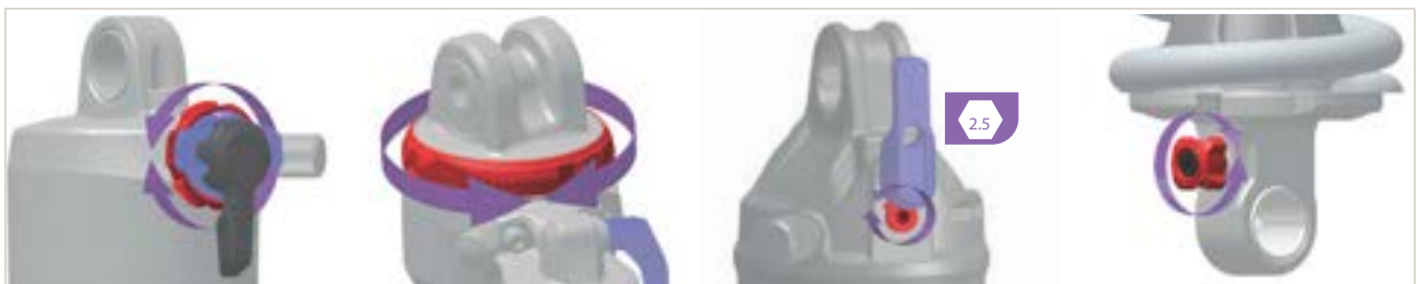
Figure 275: Position and shape of the rebound adjuster (red) depends on the model
