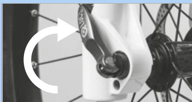
Figure 87: Closing the quick release
