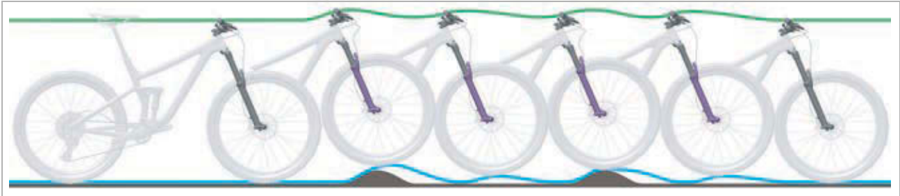
Figure 240: Suspension fork rebounding too quickly
