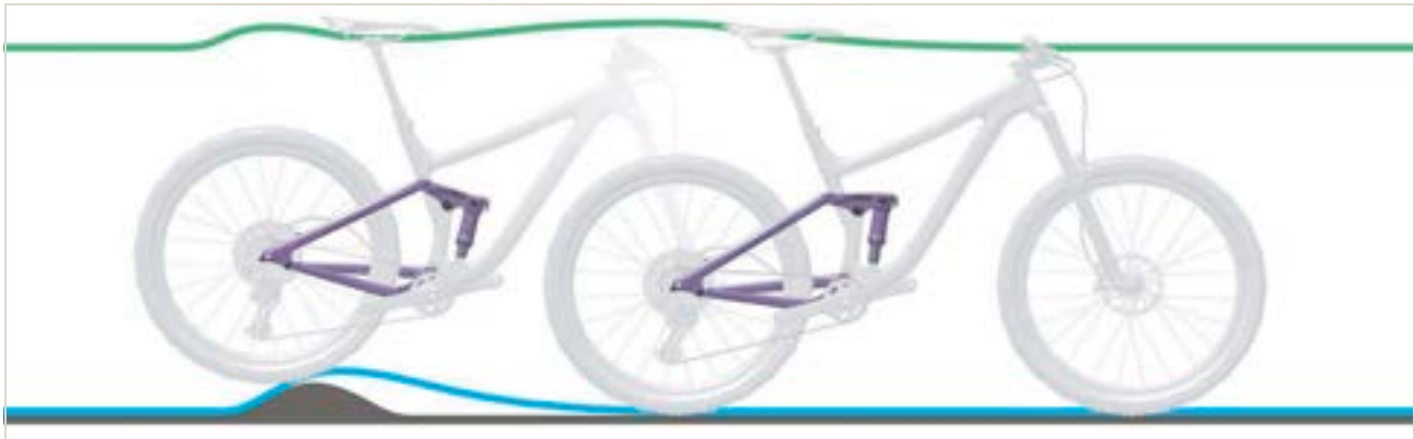
Figure 270: Excessively hard damping in the rear frame damper on bumps
