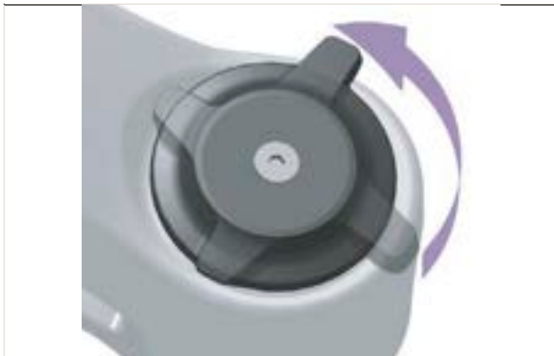
Figure 239: Adjust the compression adjuster so that it is softer
