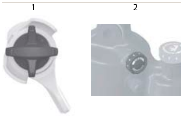
Figure 154: Float DPS (1) and Float X (2) rebound adjusters
