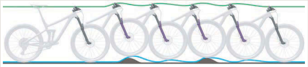
Figure 232: Suspension fork rebounding too quickly
