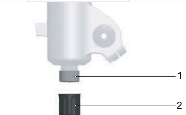
Figure 247: FOX rebound adjuster (fork) (1) under fork cap (2)
