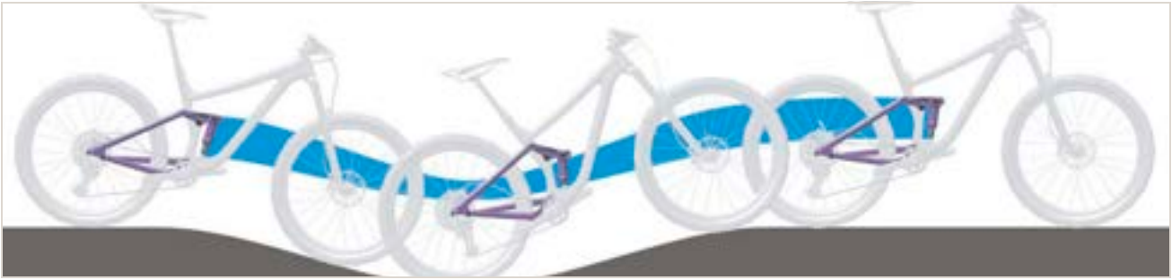
Figure 268: Excessively soft suspension in the rear frame damper on hilly terrain
