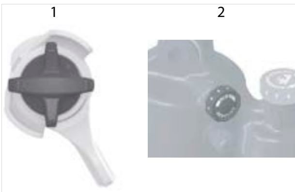
Figure 265: Float DPS (1) and Float X (2) rebound adjusters
