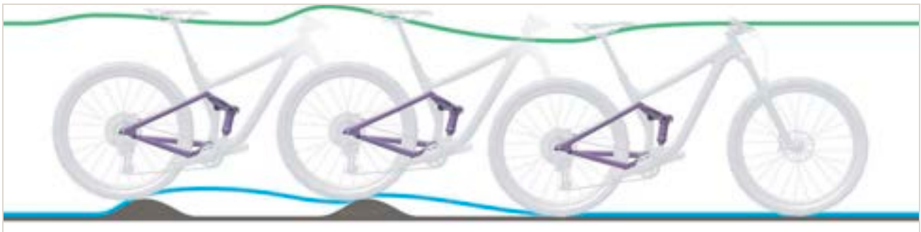
Figure 274: Rear frame damper rebounding too slowly
