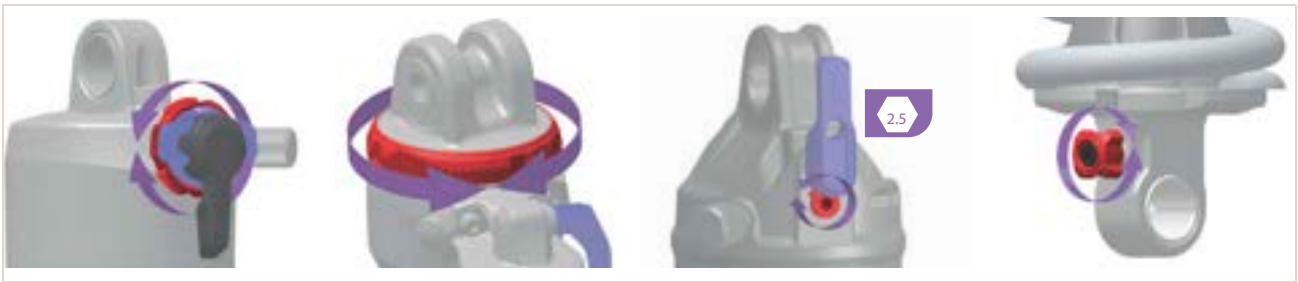
Figure 273: Position and shape of the rebound adjuster (rear frame damper) (red) depends on the model
