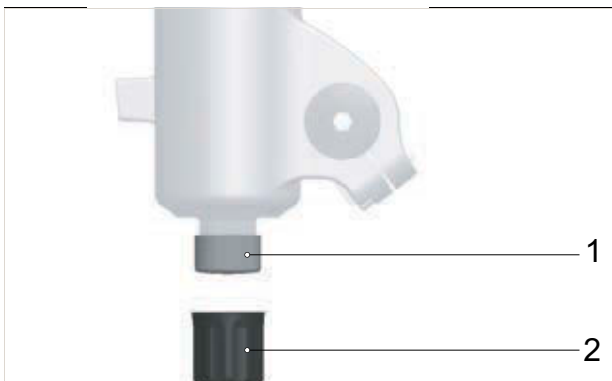
Figure 150: FOX rebound adjuster (fork) (1) under fork cap (2)
