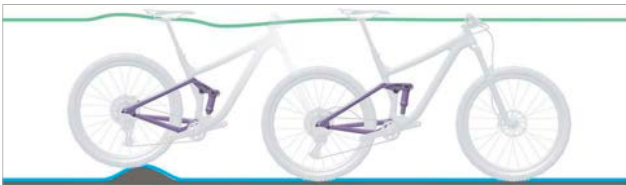
Figure 171: Optimum rear frame damper ride performance over bumps
