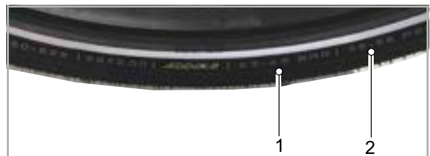
Figure 197: Tyre pressure specification in bar (1) and psi (2)
