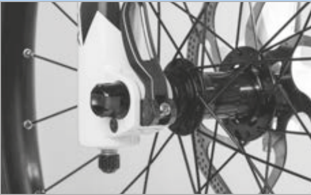
Figure 82: Perfect position for the clamping lever
