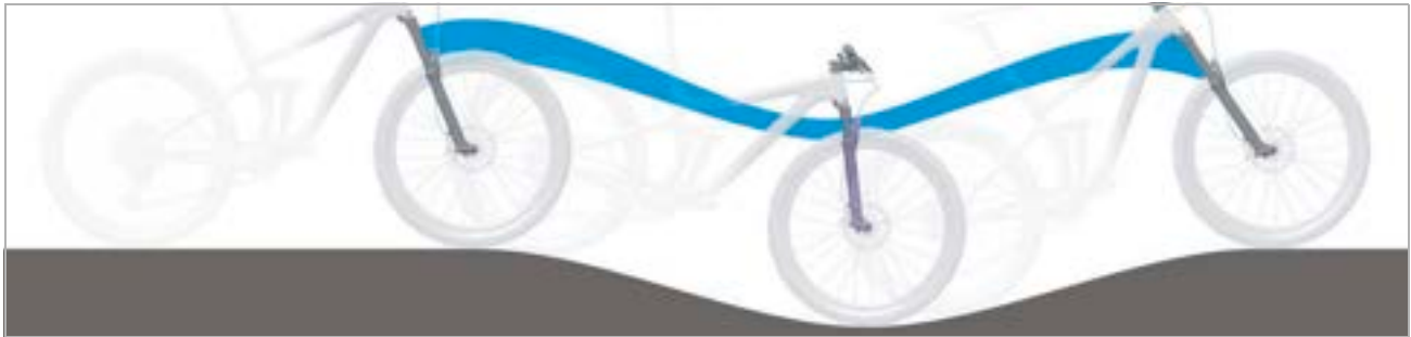
Figure 244: Excessively soft suspension in the suspension fork on hilly terrain
