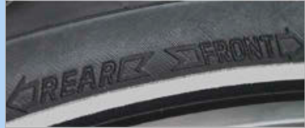
Figure 72: Rotation direction arrow on MTB tyres
