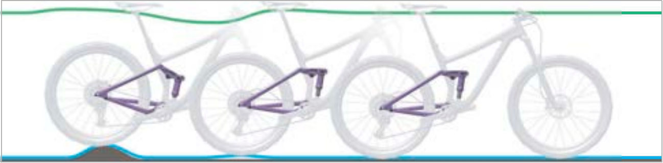
Figure 256: Rear frame damper rebounding too quickly
