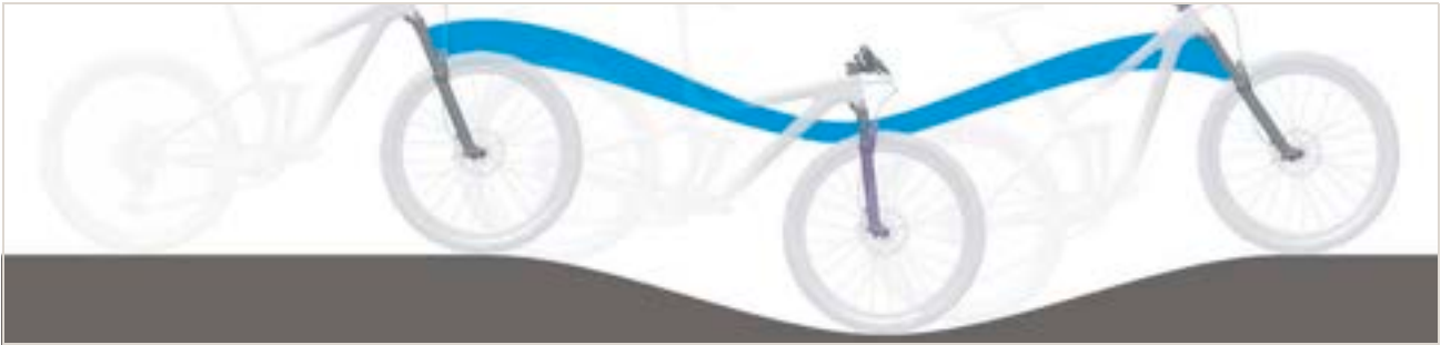
Figure 236: Excessively soft suspension in the suspension fork on hilly terrain
