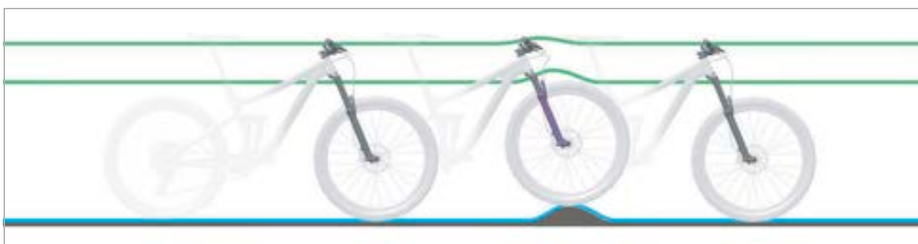
Figure 168: Compression damper set to hard and soft
