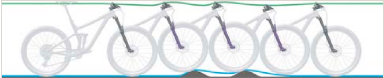
Figure 234: Suspension fork rebounding too slowly
