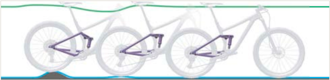
Figure 272: Rear frame damper rebounding too quickly
