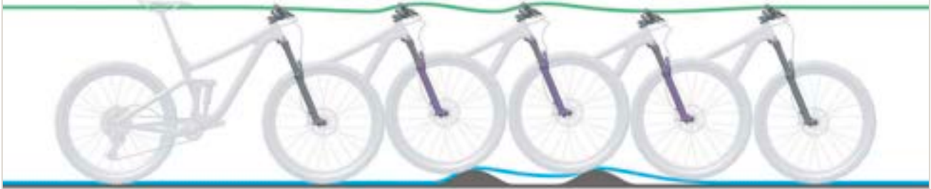
Figure 248: Suspension fork rebounding too slowly
