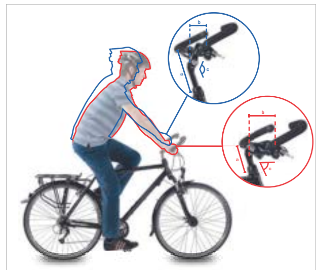
Figure 117: City bike (blue) and trekking bike position (red) by changing the angle
