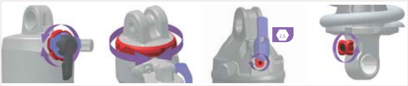
Figure 153: Position and shape of the rebound adjuster (rear frame damper) (red) depends on the model
