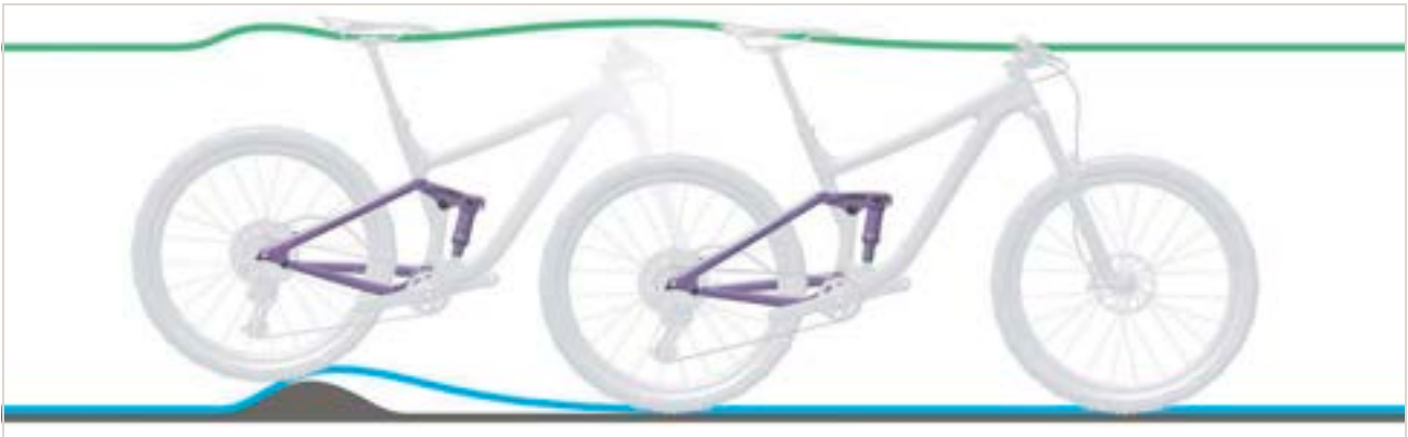
Figure 278: Excessively hard damping in the rear frame damper on bumps
