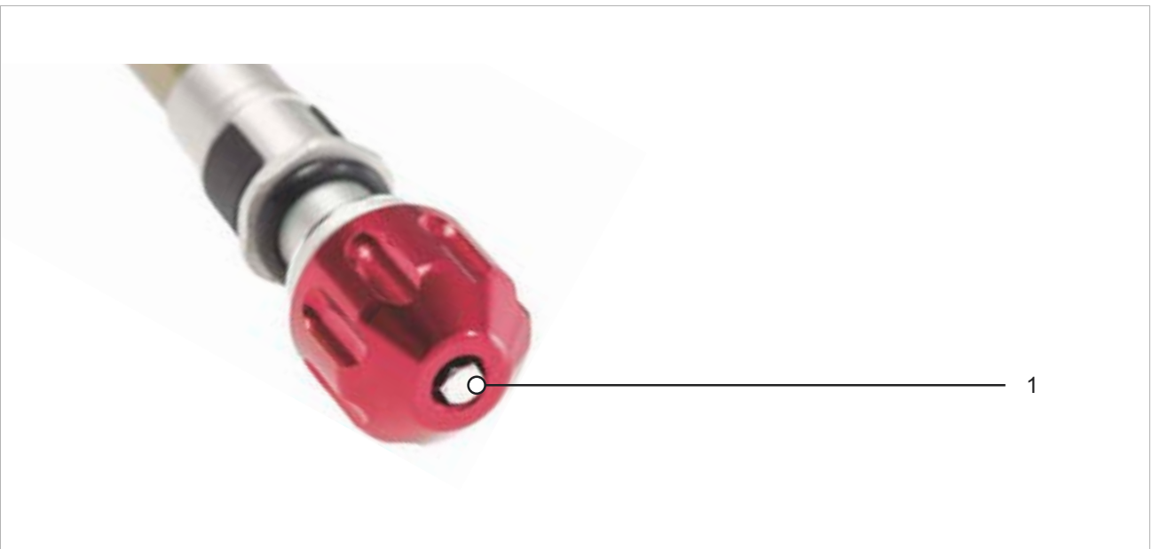
Figure 243: Example of SR SUNTOUR rebound adjuster (fork) (1)
