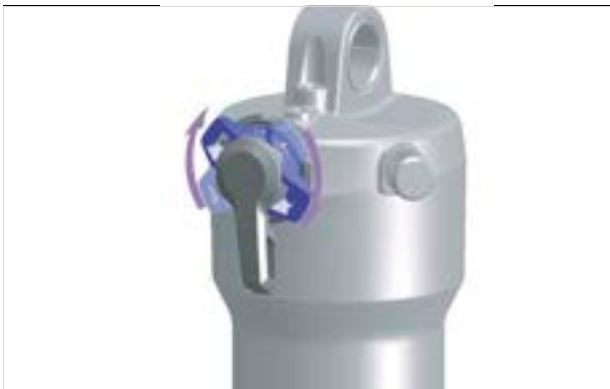
Figure 175: Adjust the compression adjuster so that it is harder
