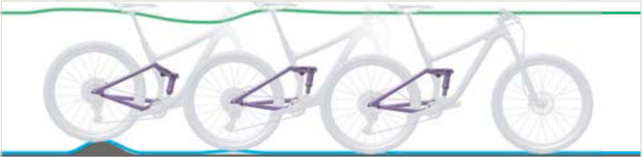
Figure 264: Rear frame damper rebounding too quickly
