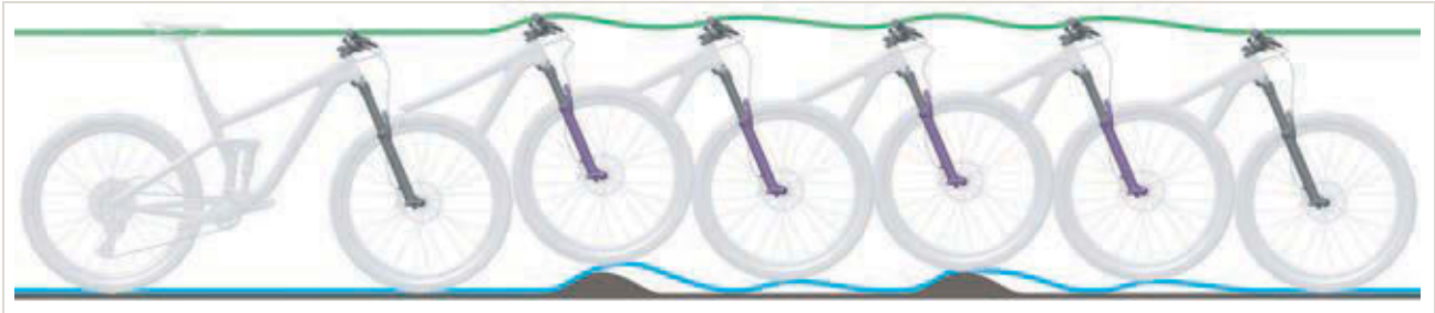
Figure 246: Suspension fork rebounding too quickly
