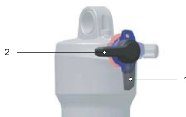
Figure 164: The compression adjuster's (black) open position (1) and threshold position (2)
