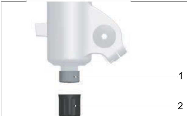
Figure 249: FOX rebound adjuster (fork) (1) under fork cap (2)
