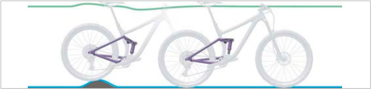
Figure 7: Optimum rear frame damper ride performance over bumps
