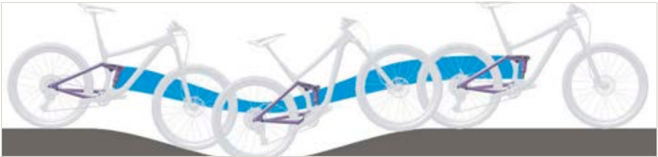
Figure 276: Excessively soft suspension in the rear frame damper on hilly terrain
