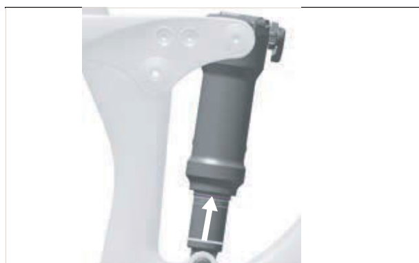
Figure 144: Moving the O-ring on the rear frame damper
