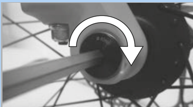
Figure 75: Tighten the axle in the direction of the arrow
