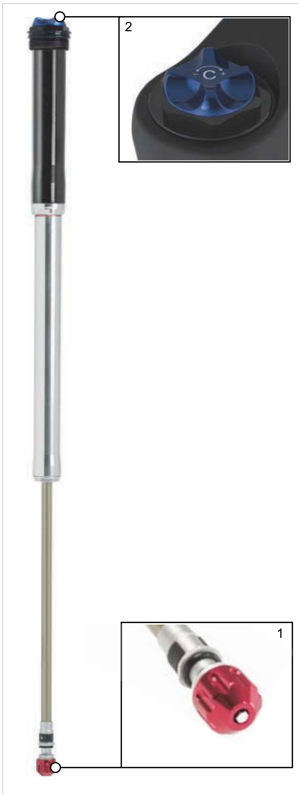
Figure 30: RC operating elements
