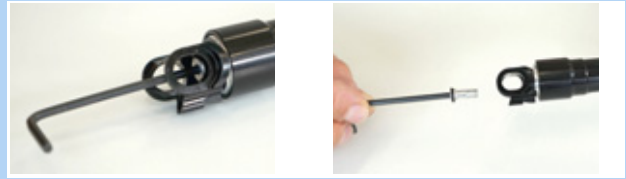
Figure 161: Unscrewing the valve cap
