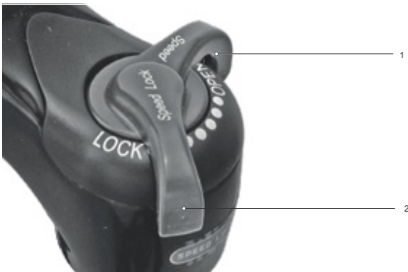
Figure 212: Changing compression adjuster to a harder setting
