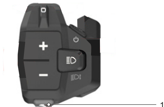
Figure 116: Position of push assist button
