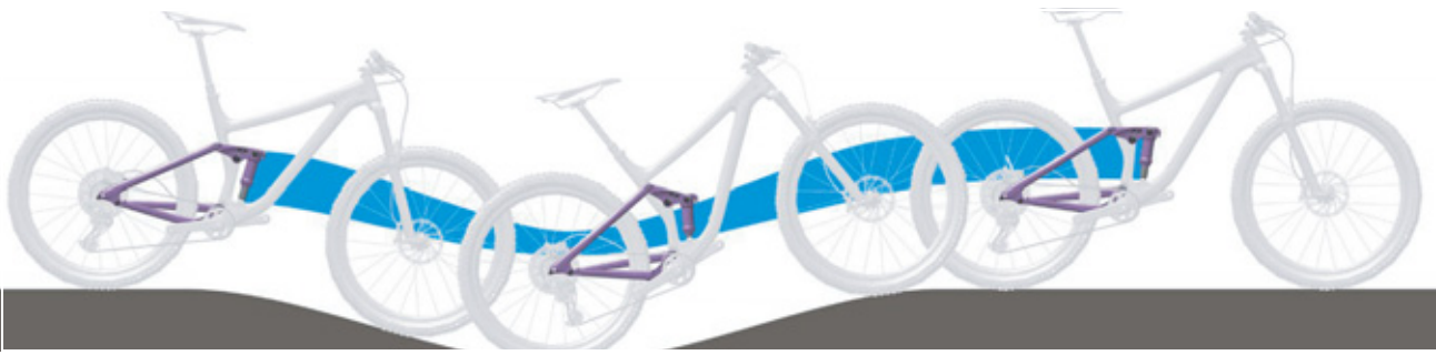
Figure 229: Excessively soft suspension in the rear frame damper on hilly terrain
