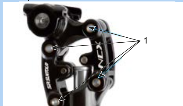
Figure 144: SR Suntour suspension seat post lubrication points
