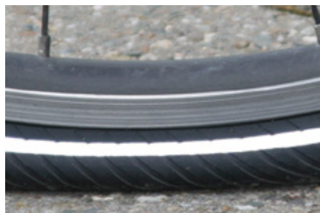
Figure 84: Much too little tyre pressure
