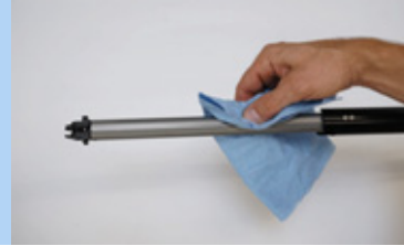
Figure 198: Cleaning the longitudinal groove
