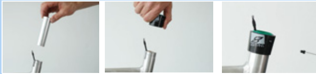
Figure 169: Fitting the slide bushing and outer sleeve
