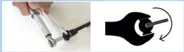
Figure 167: Setting in a clockwise direction
