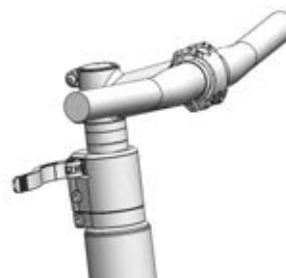
Figure 125: All Up with open stem clamping lever
