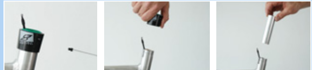
Figure 187: Removing the outer sleeve and slide bushing
