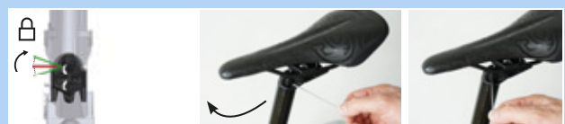
Figure 182: Closing the height adjustment
