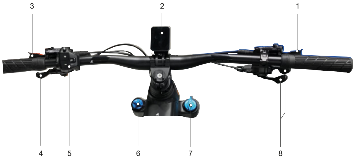
Figure 38: Detailed view of handlebars with SHIMANO SC-E800 on-board computer, used as example
