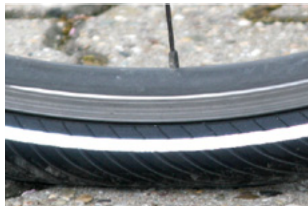
Figure 83: Correct tyre pressure. The tyre is barely deformed under the load of the body weight
