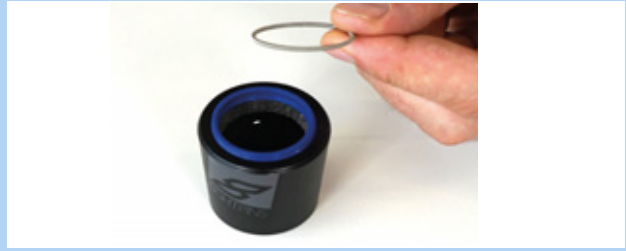
Figure 154: Removed spring washer
