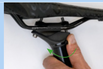
Figure 201: Closing the height adjustment
