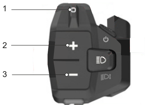
Figure 105: Position of navigation rocker switch (1), plus (2) and minus (3) buttons
