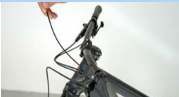
Figure 204: Attaching the end cap
